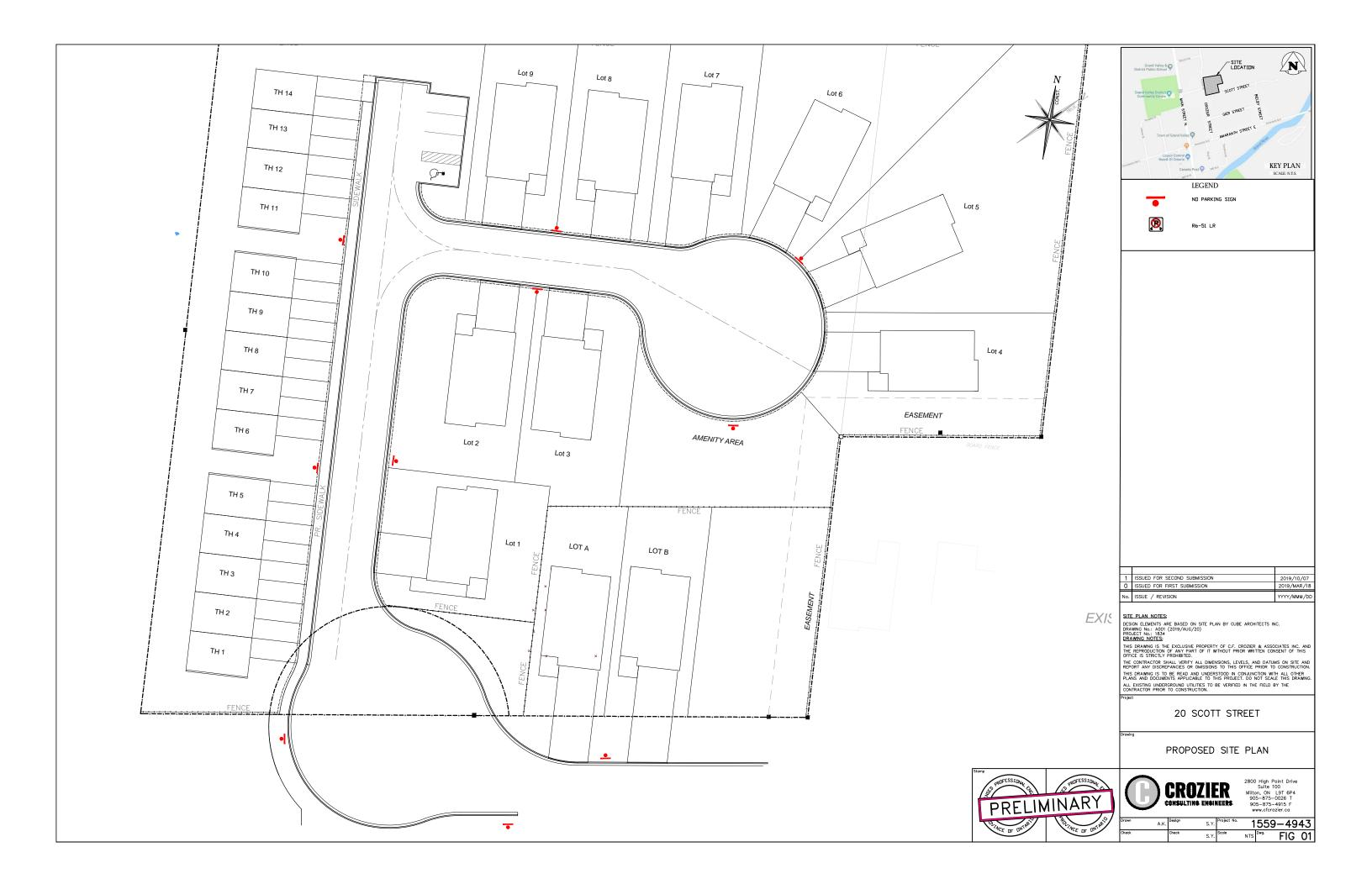
The centre line length of the primary leg of a P-loop shall not exceed 180 m. Centre line lengths shall be measured between centre line intersections of connecting roadways.
